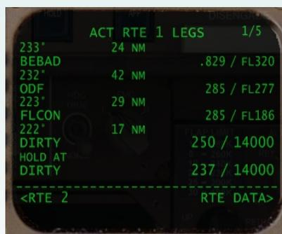
To confirm the holding pattern has been accepted, go back to the LEGS page of the FMC. As seen below, underneath DIRTY there is a “HOLD AT” qualifier.
