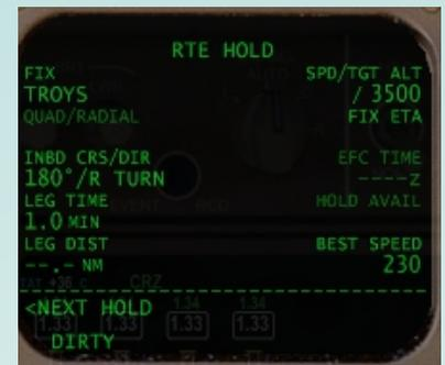
A new page appears. On the MOD RTE HOLD page, you should see your waypoint (DIRTY) at LSK 1L under FIX. Now insert the inbound course for the hold (222°). If left turns are required, type “/L” in the scratchpad and press the LSK 3L key.
