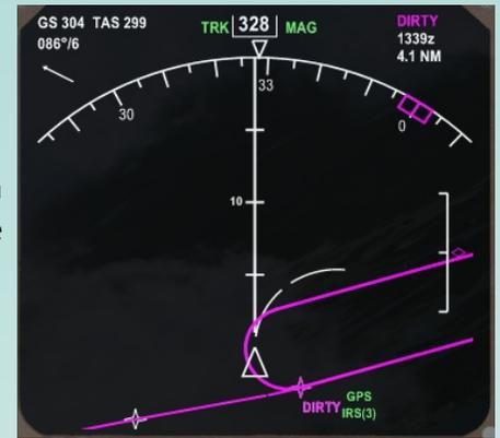
Now we are in the holding pattern and travel back in the opposite direction on a bearing of 039° for 15nm. At the end of this leg, we proceed to bank right again to come back on the original 219° heading. At this time, we have almost completed one loop. Let's assume we have now have clearance from ATC to exit the holding pattern. As we begin our approach to DIRTY for the second time, let's access the FMC. again and then press the HOLD button.
