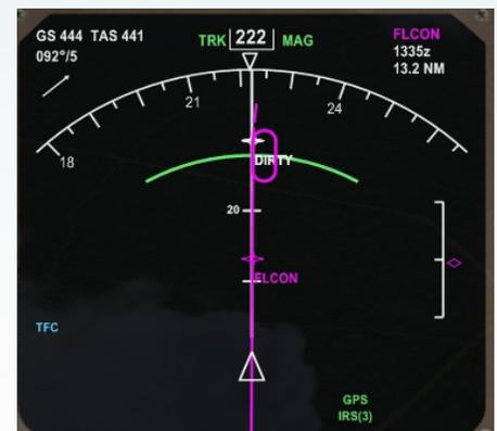
As we approach the DIRTY waypoint, we automatically begin a right turn and begin our first loop. We are still in LNAV and VNAV modes and we are positioned at 14000 and a speed of 237kts.
